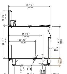
EI = Electrical inlet (power) **EQ** = Equipotential screw
